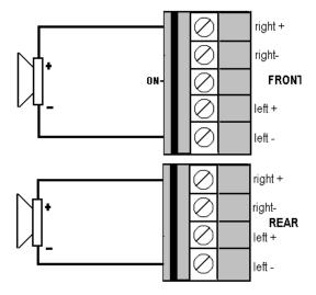
**NOTE:** For bridged two-channel operation as shown below, connect the right channel RCA cables to the Front inputs of the amplifier, and left channel RCA cables to the rear inputs of the amplifier. For summed subwoofer applications, connect the RCA cables per the input jack marking.
